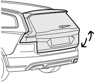
**EN** During installation on a car with automatic tailgate opener, operate the tailgate manually. Sudden and unstoppable movement of the tailgate may cause harm. Check your vehicle owner's manual for more specific information on how the automatic tailgate operates.
